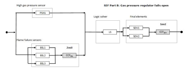
Problems with the fuel/air ratio control might be detected by measuring the gas flow and air flow. The flame failure sensor would also respond to loss of flame caused by loss of fuel/air ratio control.
